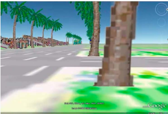
Figure 7. Real-world testing of OutRunGPS software on Balboa Island: due to limited GPS location resolution, users appeared as if they were driving through rows of trees.
