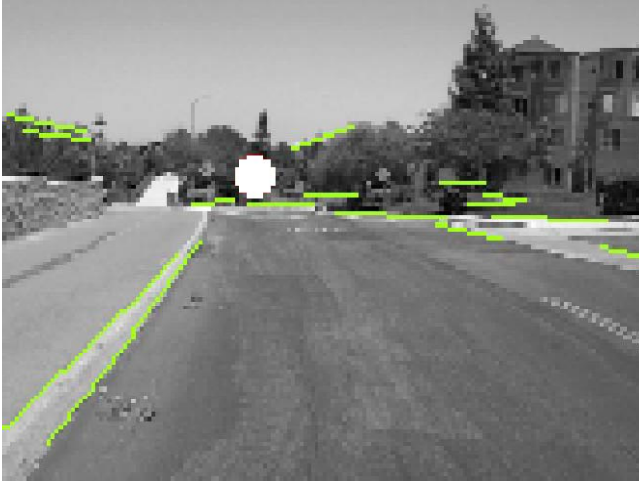
Figure 8. VPDetect processing output from cv.jit.lines to determine the road vanishing point, indicated by the white dot in the center of the image.
