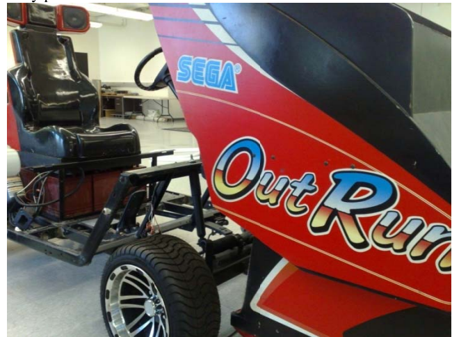
Figure 4. Physical components of the OutRun concept car: an electric golf cart and a Sega arcade game system from 1986.
